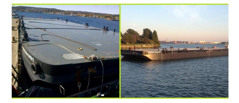
The Glovertown Spirit is a heavily constructed modern flat deck barge. Special features include a steel deck with 20 tonne per square meter deck strength. A reliable and versatile unit, the Glovertown Spirit services the Project / Transportation fleet.
