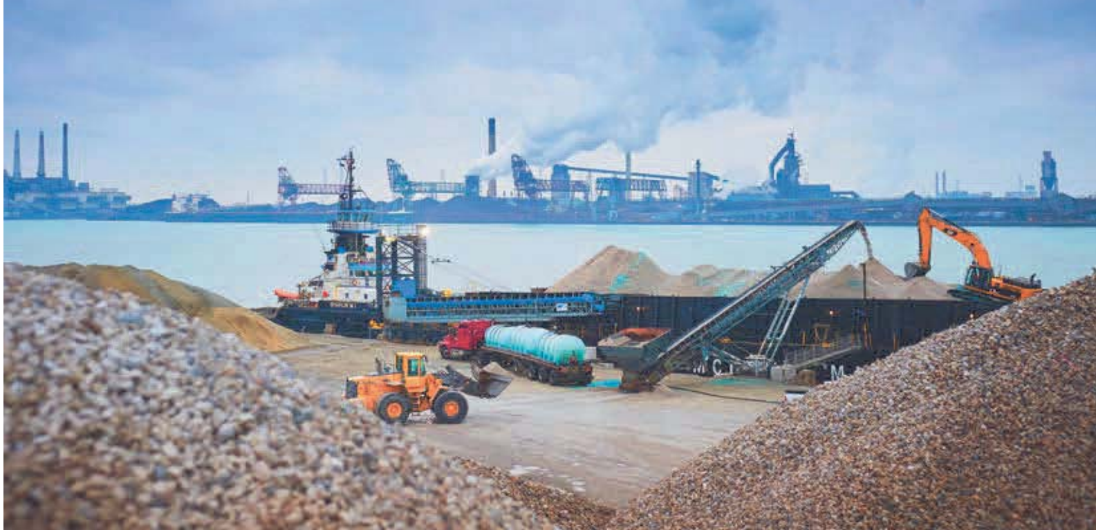
The Huron Spirit features a 150-ft self-unloading boom ideal for efficient discharge of bulk commodities. Here it is pictured unloading aggregates at the Port of Monroe.
